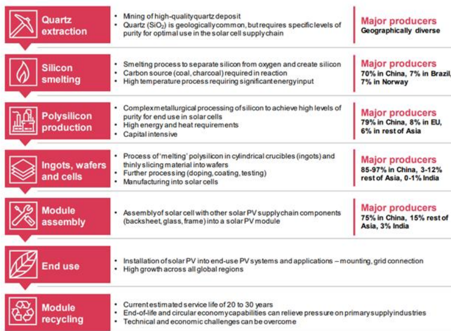
Figure 2: Solar PV supply chain (Source: CSIRO, Australian Silicon Action Plan , report prepared by PwC, November 2022).
